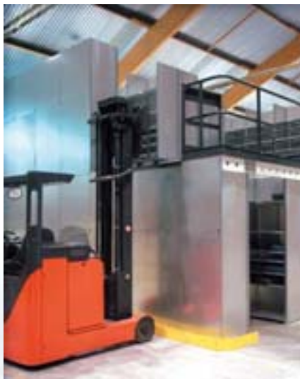
Integrated pallet gates simplify stored goods handling.
