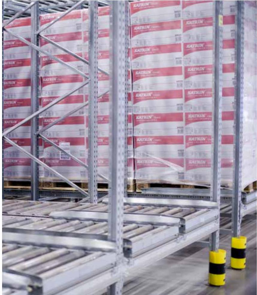
Pallet Flow Racking, or 'Pallet Live Storage' is ideal if you operate a First-in, First-out (FIFO) goods storage setup. With this system you can use up to 60% less space than if you were to use conventional pallet racking.
