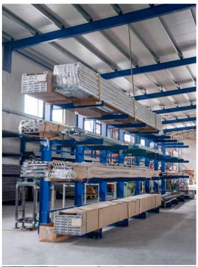
This storage system is so versatile that different component combinations can be used in various situations. The cantilever arms can be easily adjusted in height.
